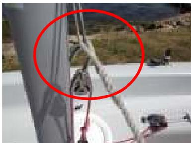
2.4 Tension the Jib until the Jib Luff (front edge) and the Shrouds are firm.
