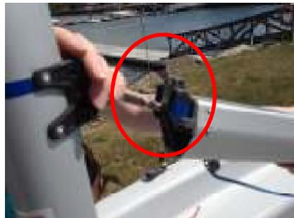
3.6 Insert the Slug (a bullet shaped object at the stern end of the sail) on the Clew of the Mainsail into the slot on the boom.
