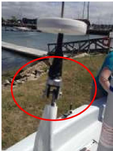
2.3 Hoist the Jib, until you can hook the jib tensioner through the loop in the wire Jib Halyard. **NOTE:** ensure that the rope tail is not trapped between the hook and the wire loop.
